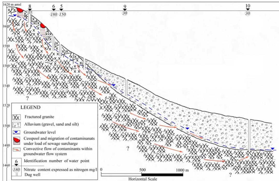
**Figure 2.** The hydrogeological cross-section of the studied area in the World Heritage Site of the St. Katherine Protectorate, showing the relative depths of wells and the convective flow of contaminants within the groundwater flow system.
