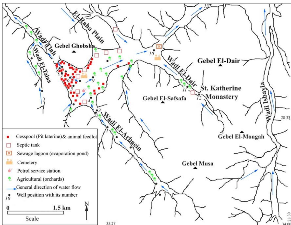
**Figure 1.** Inventory map showing location of the studied wells, potential sources of contamination and direction of flow of water in the World Heritage Site of the St. Katherine Protectorate. Wells 13 and 14 are located at 4 km and 20 km, respectively, downstream, north of well 10.
